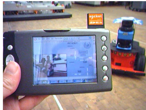
Figure 1: Pioneer AT-3 mobile robot remotely controlled by a Windows CE NET smartphone (bSquare Maui)
