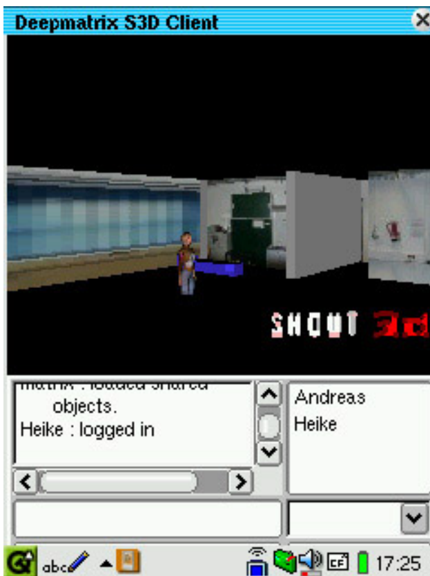
Fig. 3. Collaborative Virtual Reality environment on a Sharp Zaurus PDA, 206 Mhz ARM processor, embedded Linux, 240x320 pixel
